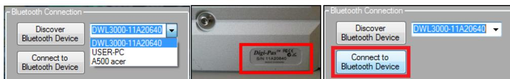
8. When the connection is established successfully, all function toolbar buttons are turned on and the status bar shows "Device Connected and DigiPas® Security Dongle is found". The DWL8500XY PC Sync is now connected to the Device and ready for use.
