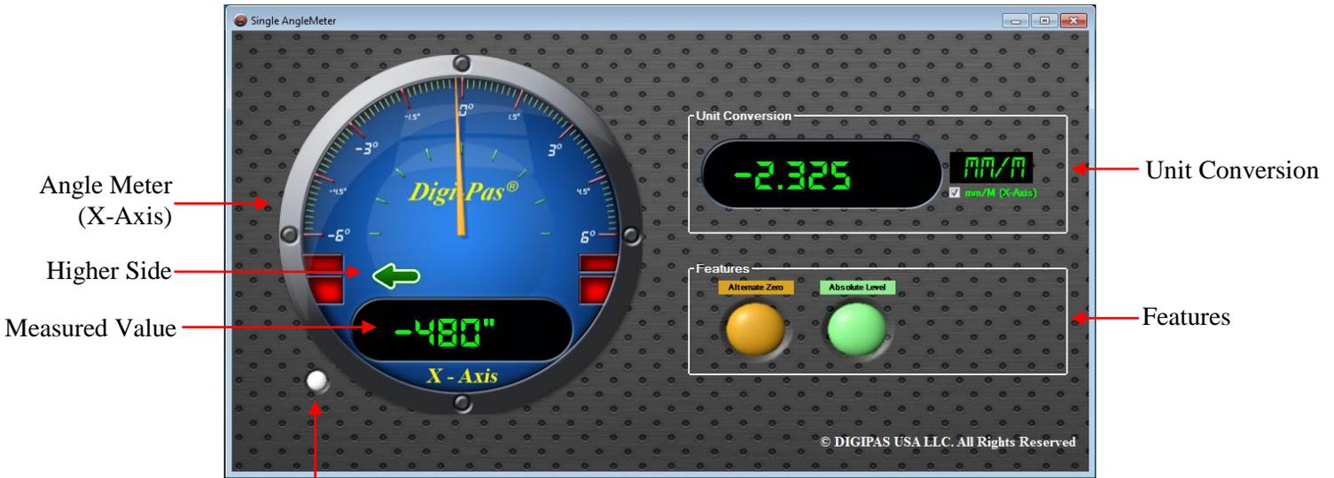
Blinking indicates measurement is in progress
