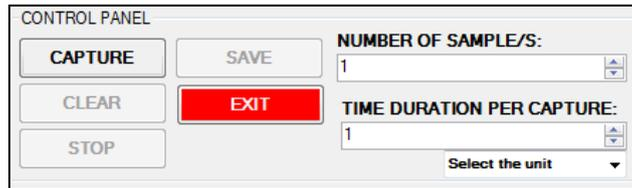
To start data logging, select the unit of time (second / millisecond). Next, select the number of samples and time duration per capture by pressing the up down arrow accordingly. Click CAPTURE button to initiate data logging. Click STOP button to halt data logging and click CLEAR button to erase or click SAVE button to store the data. EXIT button is used to quit the Dual Angle Graph window.
