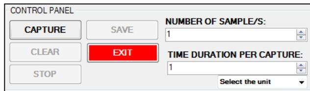
To start data logging, select the unit of time (second / millisecond). Next, select the number of samples and time duration per capture by pressing the up down arrow accordingly. Click CAPTURE button to initiate data logging. Click STOP button to halt data logging and click CLEAR button to erase or click SAVE button to store the data. EXIT button is used to quit the VibroMeter window.
